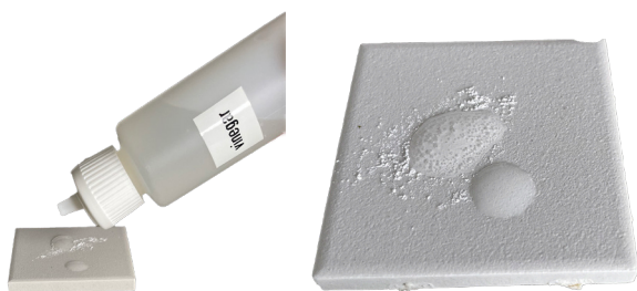
acid test with vinegar
