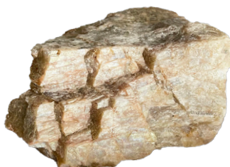
a platy cleavage with one plane of weakness
